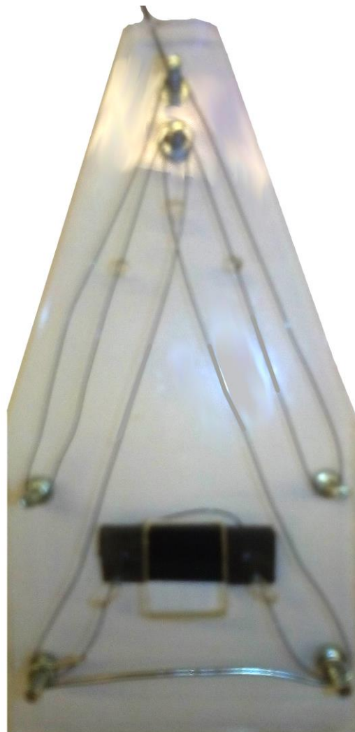
Figure 64: Bottom view of the PMMA wire base for the finger compressor, with SMA wire wrapped around the screws. Voltage was applied between the steel wire at the bottom of the image (ground) and the screw at the top. The black ABS in the middle serves as shielding.
