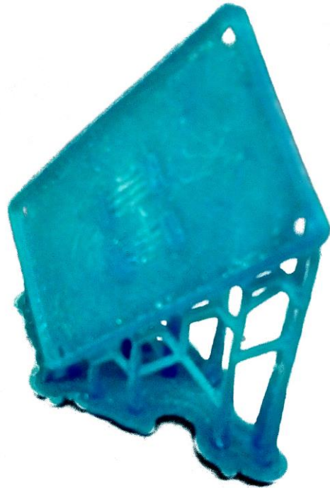
Figure 11: A base part printed with a “high-precision” resin, but not flat on the build plate as intended.
