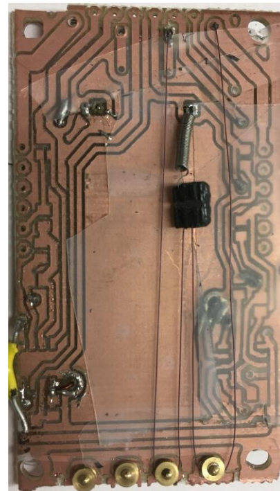
Figure 39: Bottom side of the milled PCB with one actuator cell attached. Transparent tape isolates the SMA wire from the board. All pulleys are isolated.
