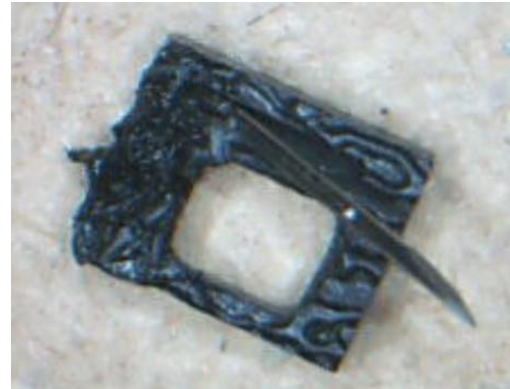
Figure 54: Bottom view of the (5-mm-long) milled lancet holder with the lancet inserted. The melted-over trench holding the driven shank is on the left.
