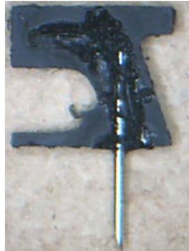
Figure 62: Physical implementation of the lancet holder of Fig. 57 for the spring-loaded actuator concept. Trench melting was difficult at this scale, but the resulting lancet fixture was firm.
