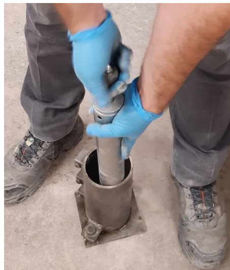
Figure 3.5. Using standard proctor hammer for the compaction of concrete mixtures.
