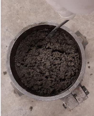
Figure 3.6. Scratching the top surface of each layer to create better bonding between the layers.
