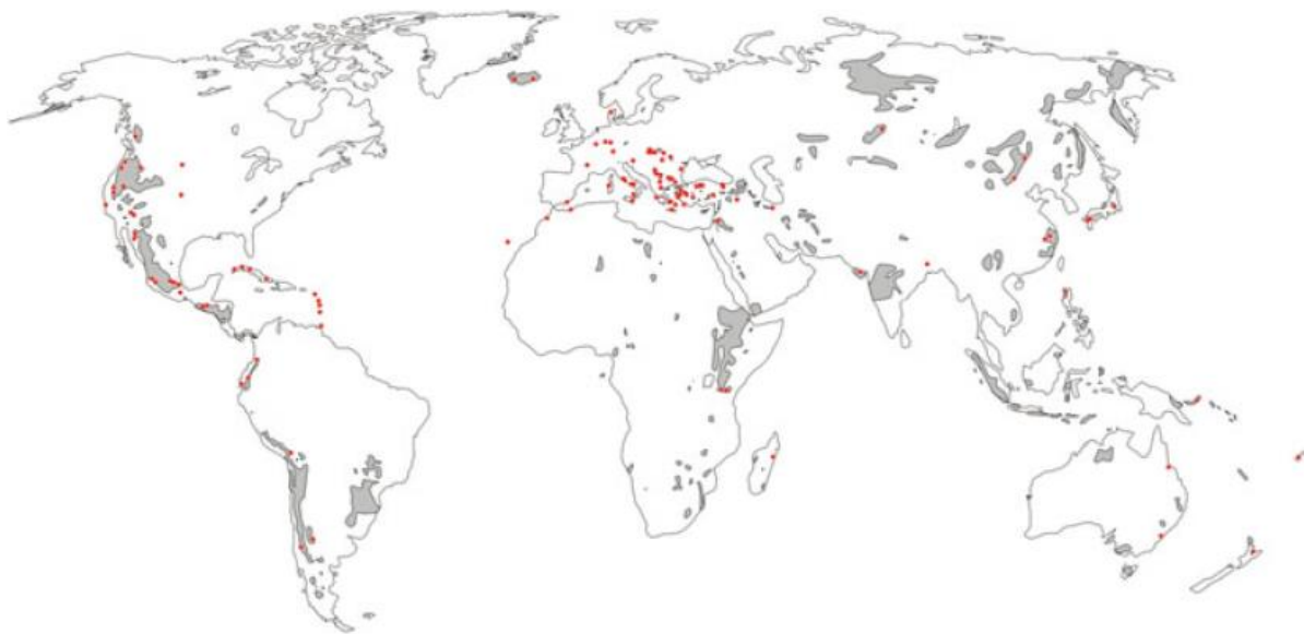
Figure 2.2. Global distribution of volcanic rocks (grey regions) and reported natural pozzolan deposits (red dots) [54].
