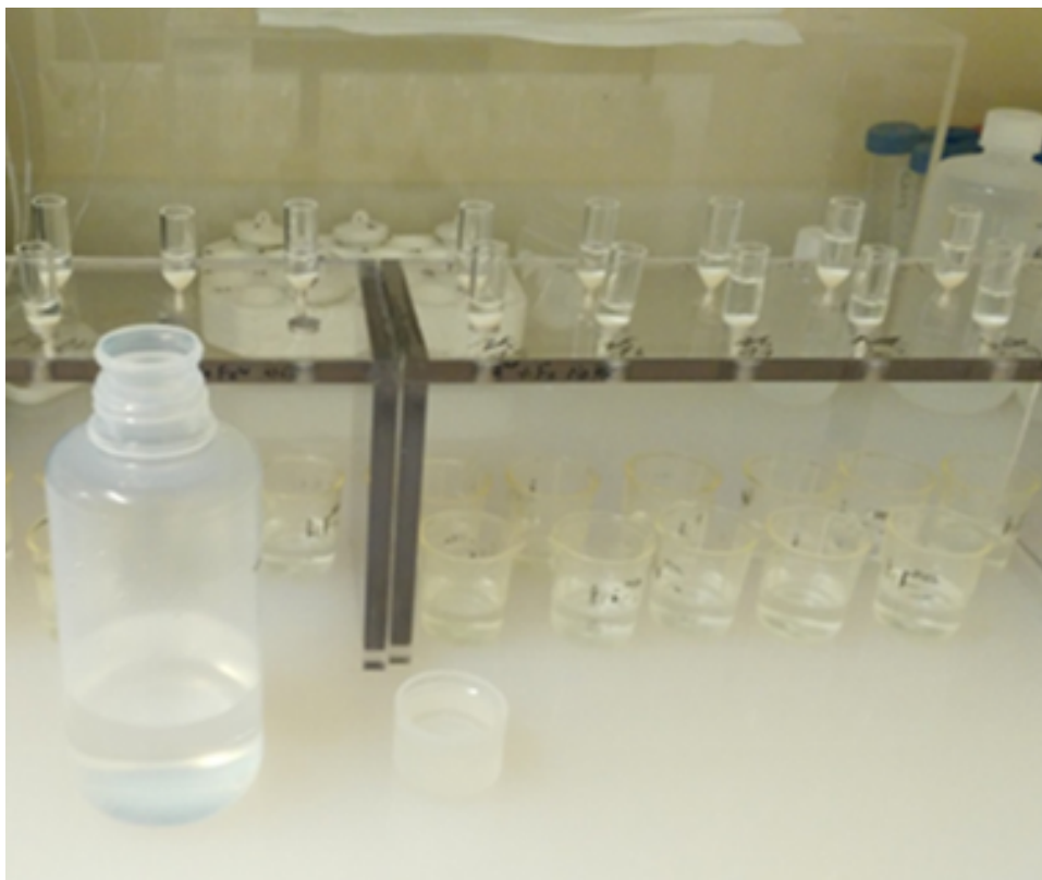
Figure 3.2: An ion exchange setup for sample preparation in isotopic analysis
