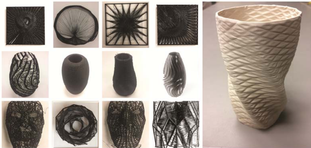
Figure 37. Surface effects created through 3d-printed glitches
