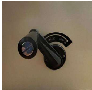
Fig. D.3 Unloading and Loading position
