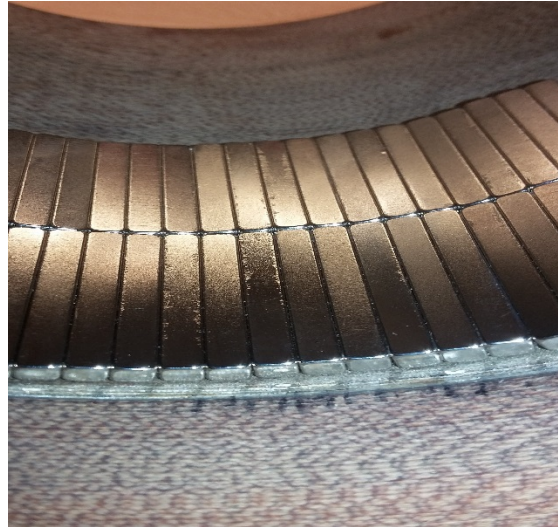
Figure 4-10 The inner side of the inner rotor with magnets
