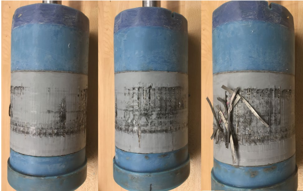
Figure 5- 26 The modulating ring damage from all the sides
