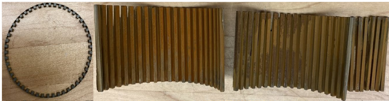
Figure 5-10 Water-jet cut modulating ring
