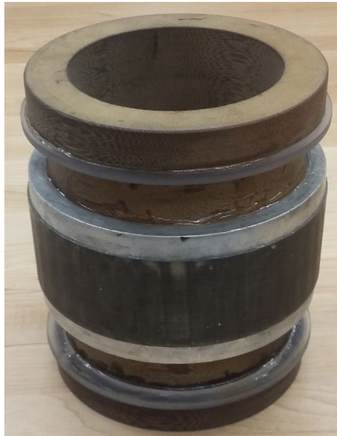
Figure 4-9 Outer rotor with micarta parts
