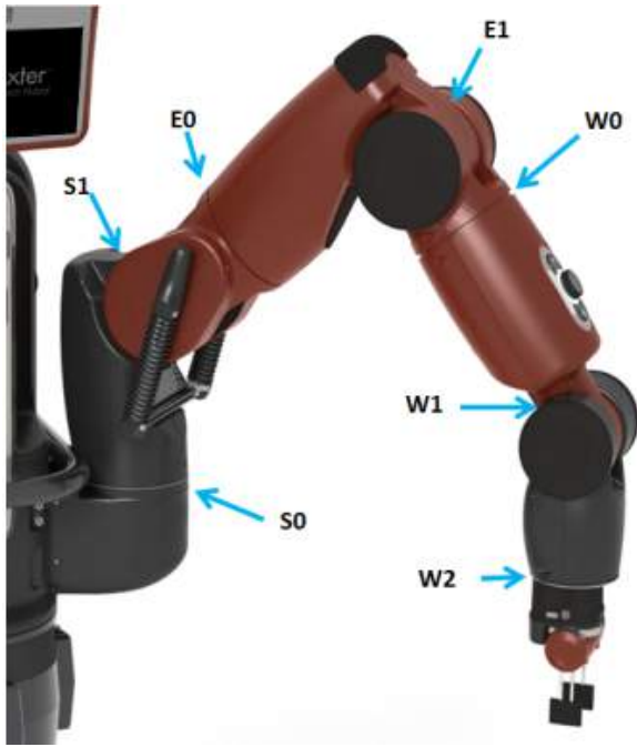
Figure 3: Diagram of Baxter's seven degrees of freedom and joint names
