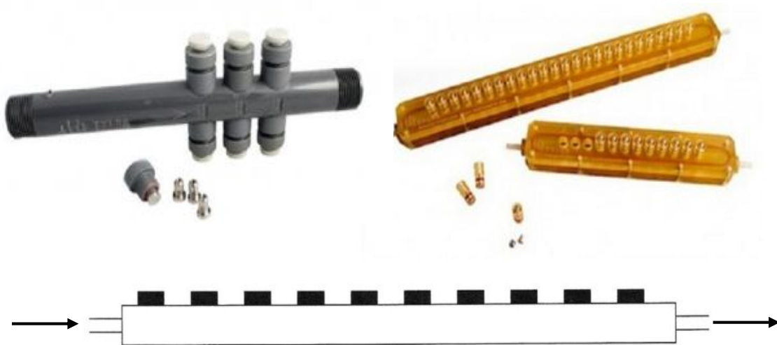
Figure 1.11 Robbins device used to establish SRB biofilms in souring control studies. (Pictures are from Tyler Research Corporation: http://www.tylerresearch.com )
