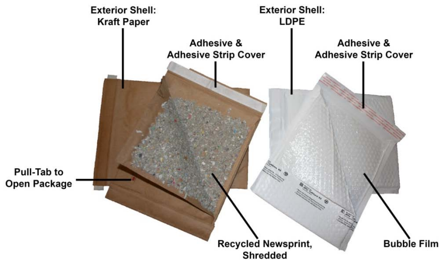
Figure 6: Self-sealing Protective Mailer Components: Kraft padded mailer (left) made from 50% post-consumer paper and LDPE bubble mailer (right) made from co-extruded LDPE
