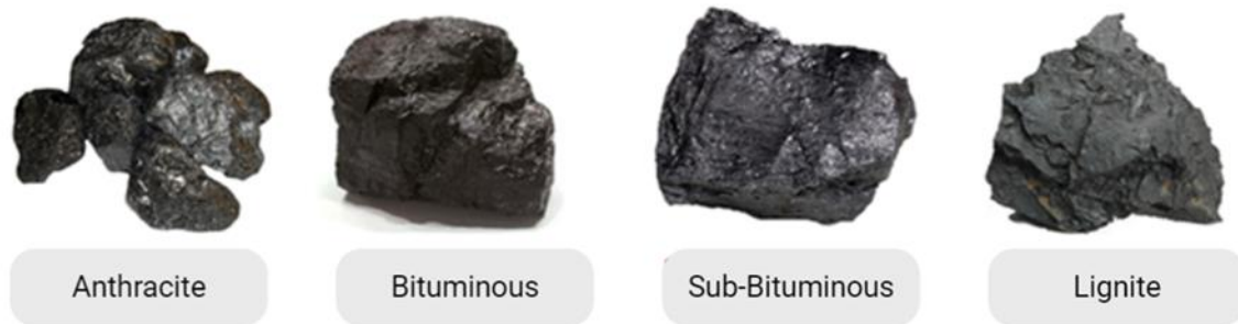
Figure 2.1: The different types of coals arranged based on rank starting with the highest rank anthracite coal.
