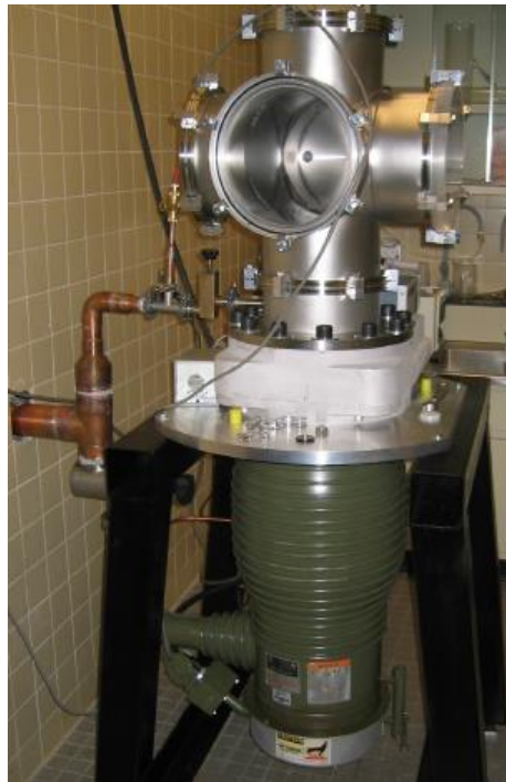
Figure 3-3: Photograph of the vacuum system showing the six-way vacuum chamber, diffusion pump, and the pneumatic gate valve in the middle.
