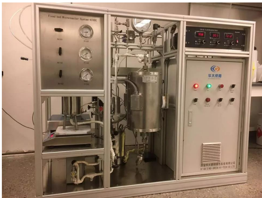
Fig. 2.1 fixed-bed reactor used for methane-assisted desulfurization and deoxygenation studies
