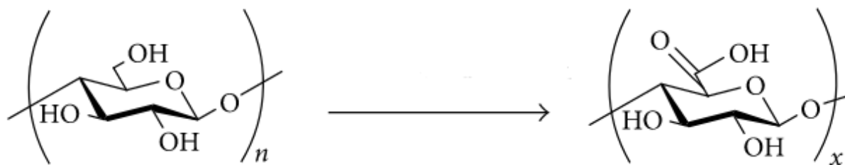
Figure 2-5 Cellulose oxidation to 2,2,6,6-tetramethyl piperidine-1-oxyl, radical (TEMPO)-oxidized cellulose nanofibers (TOCN) (Kotatha and Rungrodnimitchai, 2018).
