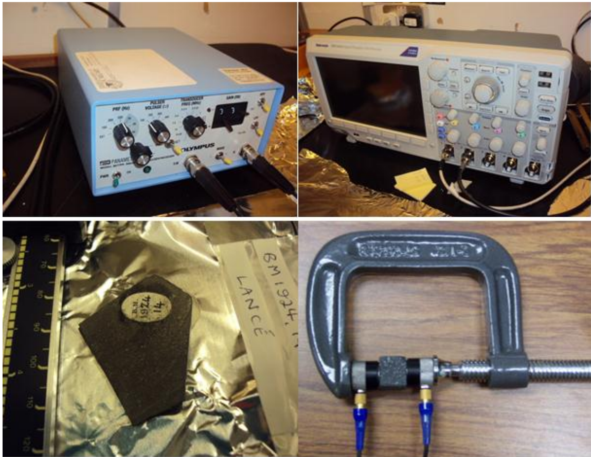
Figure (3.5): Shows images of the equipment used throughout the elastic wave velocity measurements: A manually controlled electric pulse generator/receiver (Olympus Model 5077 PR) with a bandwidth of 35 MHz (Upper left), a 100-MHz-bandwidth Tektronix Digital Phosphor Oscilloscope Tektronix Model DPO2014 (Upper right), a sample slab of Lancé (CO-chondrite), two pairs of 6-mm-diameter P- and S- wave ultrasonic contact transducers (Olympus V133 and V156 respectively) and a pair of C-clamps.
