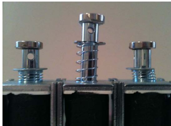
Figure 5.2 Inactive (lowered) and active (raised) permanent switchable magnets used to create magnetic tactile pixels in the Fuse-Map prototype system
