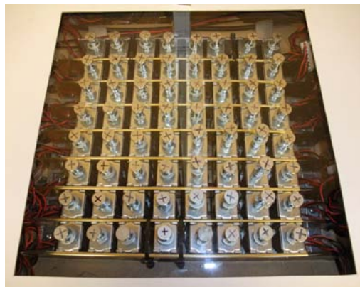
Figure 5.10 The Fuse-Map interface's magnetic tactile display device.
