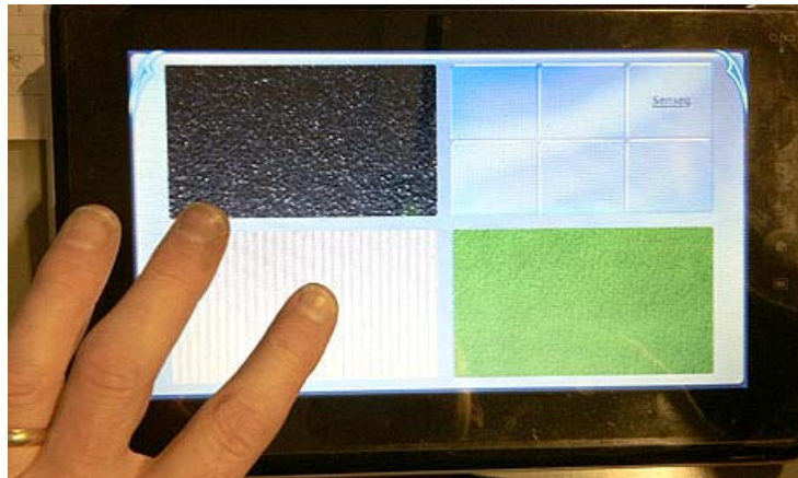
Figure 3.10 Senseg E-Screen device demonstrating different tactile sensations such as grit, ridges, corduroy and leather (Arthur 2012).
