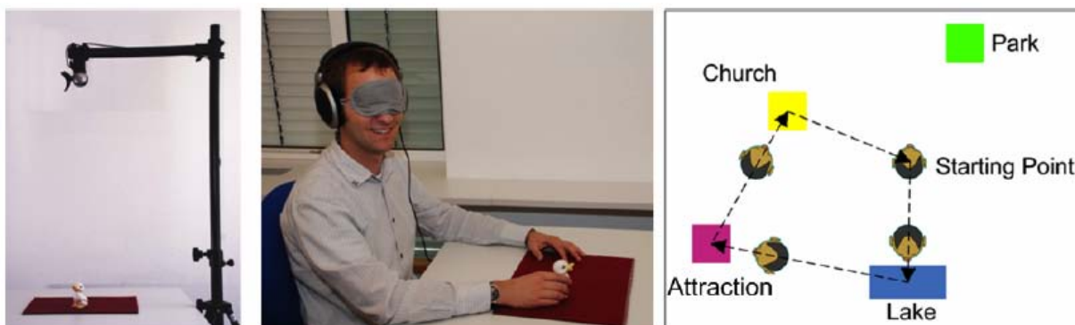
Figure 3.5 Participant demonstrating the use of Pielot et al's (2007) motion capture and artefact based auditory mapping system. This figure depicts a motion capture apparatus used to track the position of the interface avatar (left), a user exploring a map scene by moving the interface avatar (centre), and a rendering of the user's movement within the virtual map scene (right).
