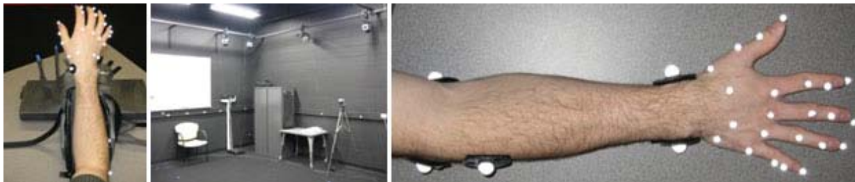
Figure 4.5 Visible Light Markers used for Hand Tracking (Rahmatalla 2012).
