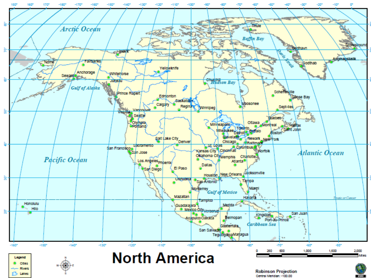
Figure 4.6 A sample map illustrating basic map elements such as titles, labels, borders, graticules, neat lines, scale bars, north arrows and orientation references, legends, captions, metadata, and publishing references (ESRI 2008).
