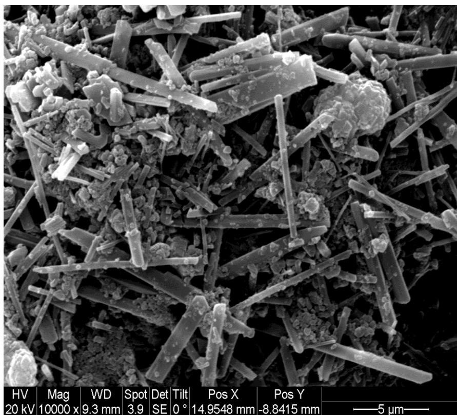
Figure 2.5. SEM image demonstrating the homogeneity of a sample of MOF-74-A.
