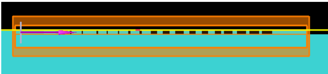
Figure 7.16: Output grating schematic from Lumerical. Purple arrow signifies the mode source, bright yellow line above gratings indicates power monitor
