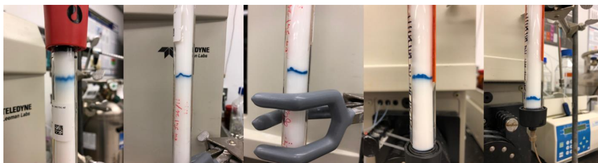
Figure 3.4: Image of the surface of the column bed after five injections of unfiltered rabbit plasma and one injection of blue dextran. A yellow discolouration and black solids are clearly visible.
