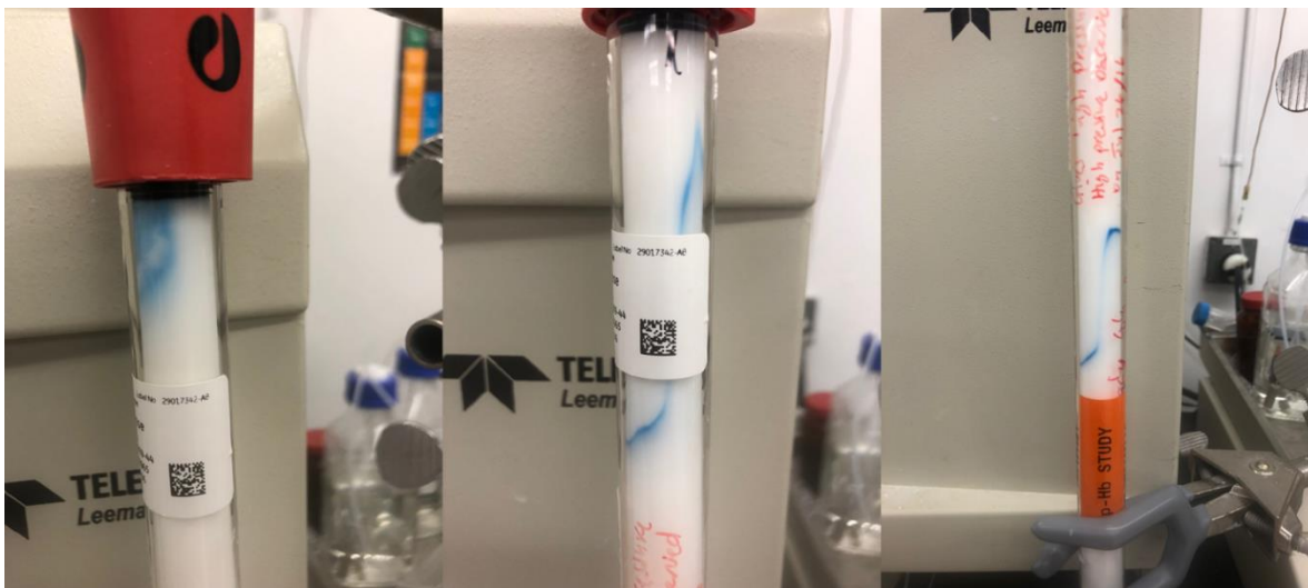
Figure 3.3: Image of non-uniform blue dextran dye migrating through the SEC column after the column performance has been adversely affected by five subsequent injections of unfiltered rabbit plasma.
