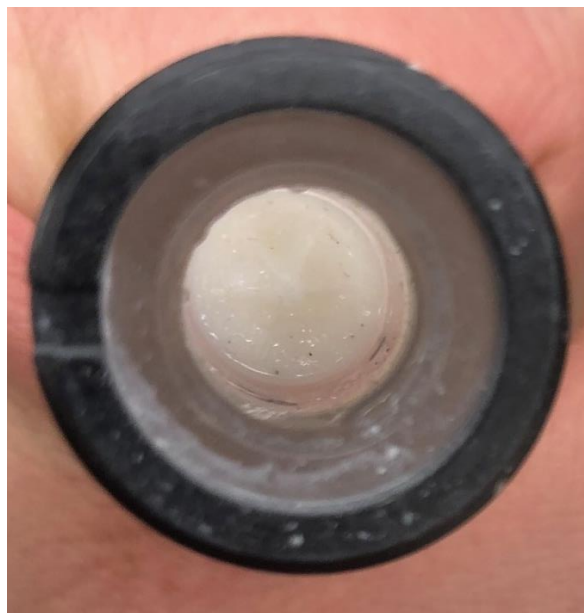
Figure 3.4: Image of the surface of the column bed after five injections of unfiltered rabbit plasma and one injection of blue dextran. A yellow discolouration and black solids are clearly visible.
