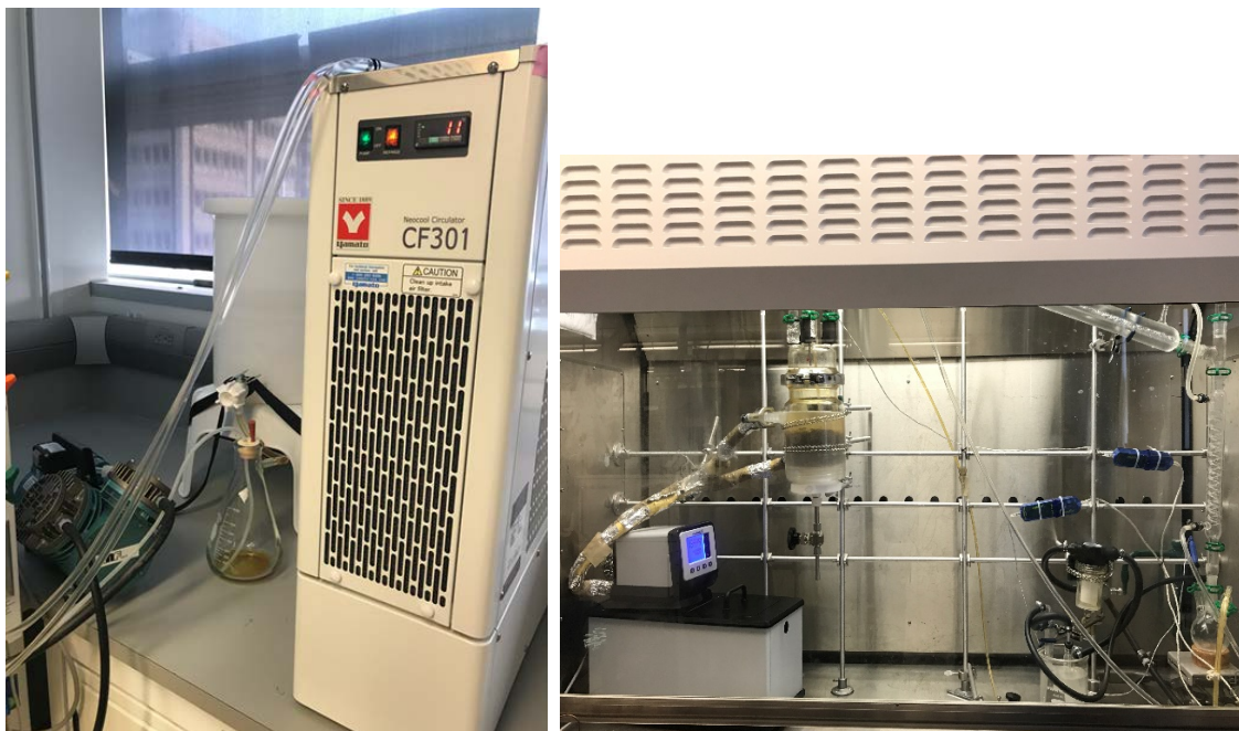
a) the vacuum pump, cooling system and feed tank b) principal part of reclaimer
