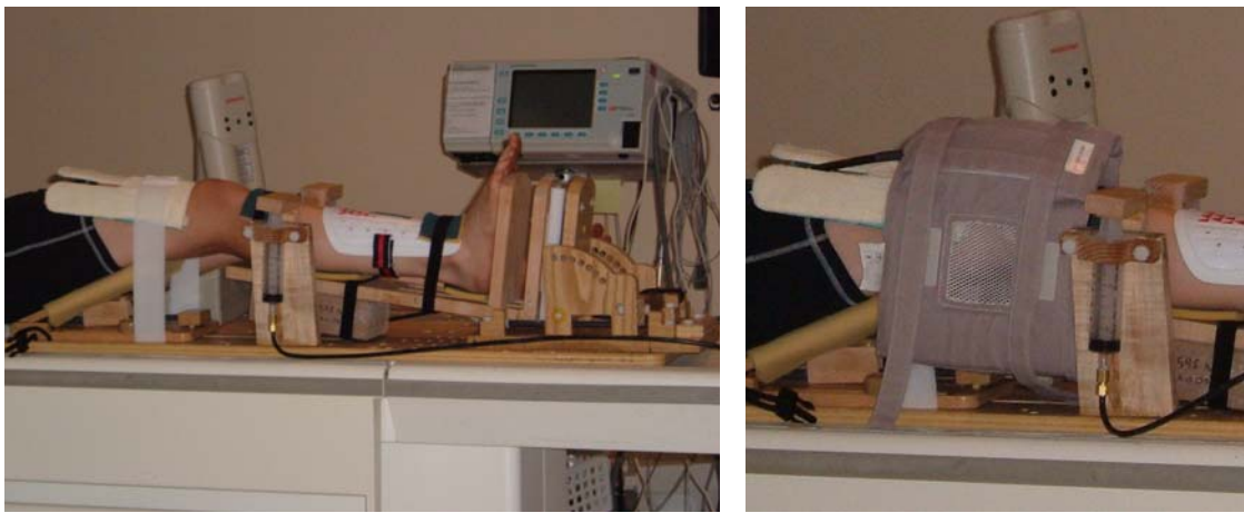
(a) (b) Figure 4-3: MR Imaging test setup (a) prior to and (b) after adding the flex coil
