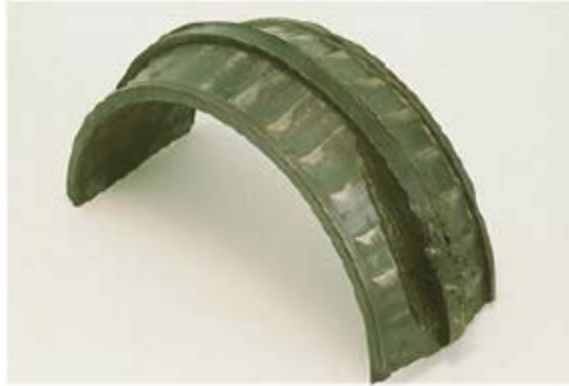
Figure 2.7 Bearing seizure failure (Courtesy of Emerson Bearing)
