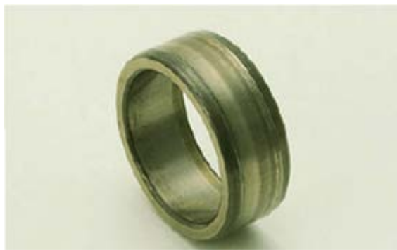
Figure 2.4 Bearing wear failure (Courtesy of Emerson Bearing)
