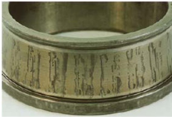
Figure 2.5 Bearing corrosion failure (Courtesy of Emerson Bearing)
