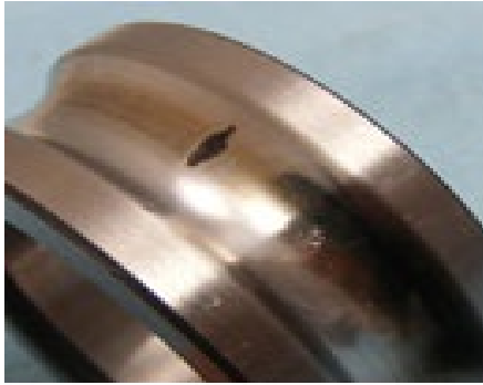
Figure 2.3 Bearing pitting failure (Courtesy of JAD Associates)
