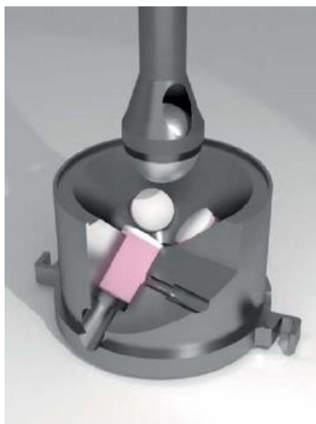
Figure 2-1. Schematic illustration of tribological set-up of three cylindrical samples with a spherical probe. Adapted from [21].
