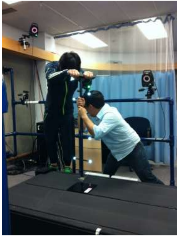
Figure B-1. MTD-2 calibration rod and an illustration of the calibration procedure.
