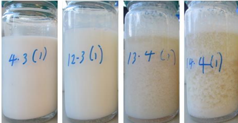
Figure 4.6 Pictures of emulsions with HLBs of 4.3, 12.3, 13.4 and 14.4 immediately after mixing showing no phase separation for HLB 4.3 and 12.3 while showing phase separation for HLB 13.4 and 14.4
