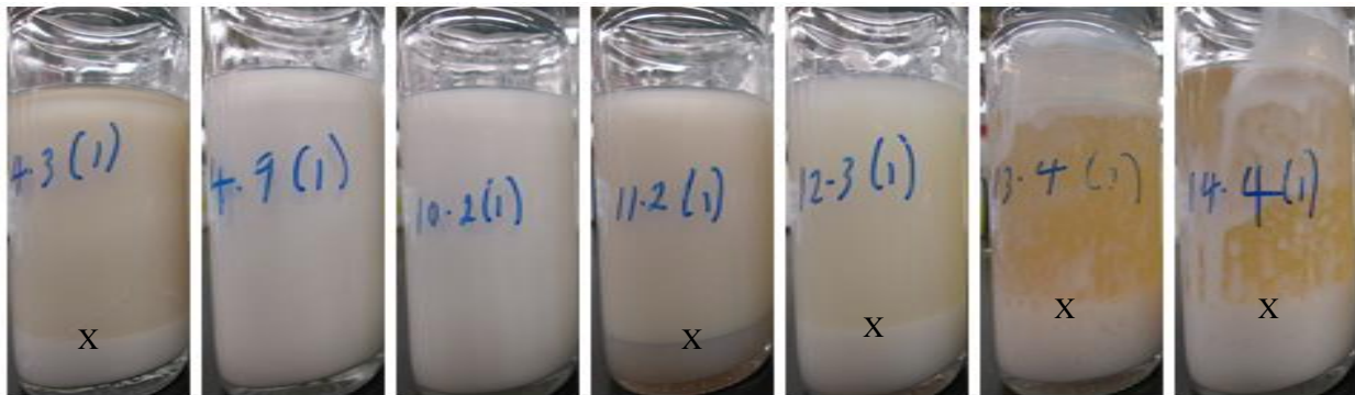
Figure 4.7 Pictures of emulsions with a range of HLB values after 24 hour aging showing phase separation for HLB 4.3, 11.2, 12.3, 13.4 and 14.4 (X) while no phase separation for HLB 4.9 and 10.2
