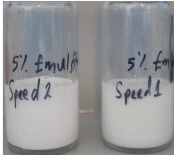
Figure 4.2 Pictures of emulsion obtained after 24 hour static aging of emulsions with 5 % emulsifier (A) blend showing no phase separation
