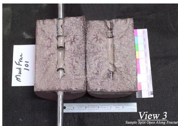
Figure 7: A split core sample during GPRI 2000 tests 9
