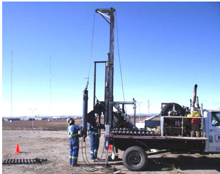
Figure 3-1: Waste drilling and sampling at Shepard landfill site
