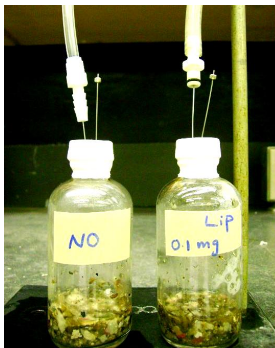
Figure 4-1: Nitrogen purging into batch reactors
