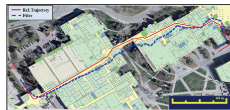
FIGURE 8: PDR trajectory compared to a reference trajectory.
