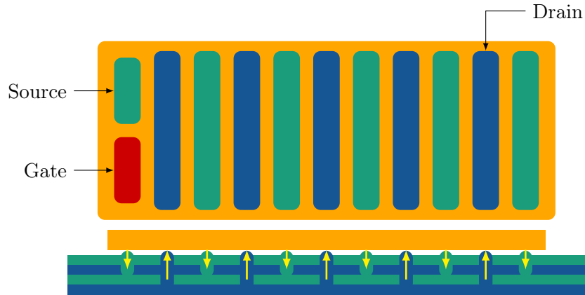
Figure 1.3: LGA package template of GaN E-HEMT by EPC. Alternating the PCB layers between source and drain increases the exposure of reverse currents causing the magnetic fields generated to cancel out while also sinking heat into the PCB.
