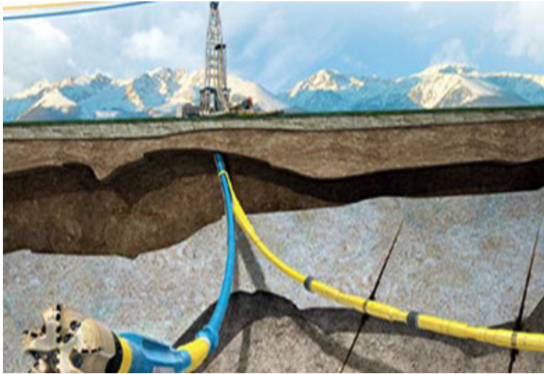
Figure 1.1: Schematic of directional drilling (Discovery Channel Online, 2011)
