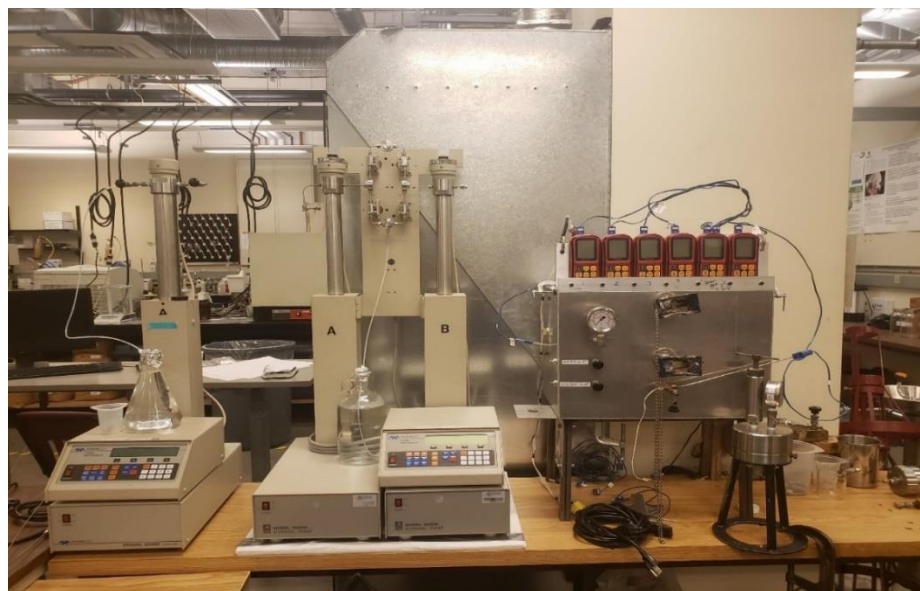
Figure 3.2: Experimental setup for SAGD and SA-SAGD experiments.
