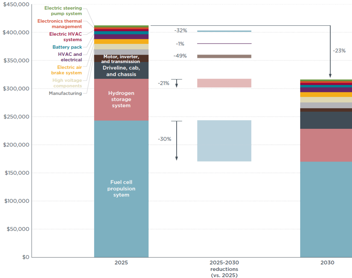
Fig. 4.5. Example of Estimated Cost Reductions for Hydrogen Fuel Cell Tractor Truck Components in 2030 and the Estimated Composition of Costs in 2030. Figure taken from Figure 6. from (Sharpe and Basma, 2022).
