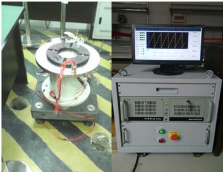
Figure 4.24 Single-axis rotation platform
