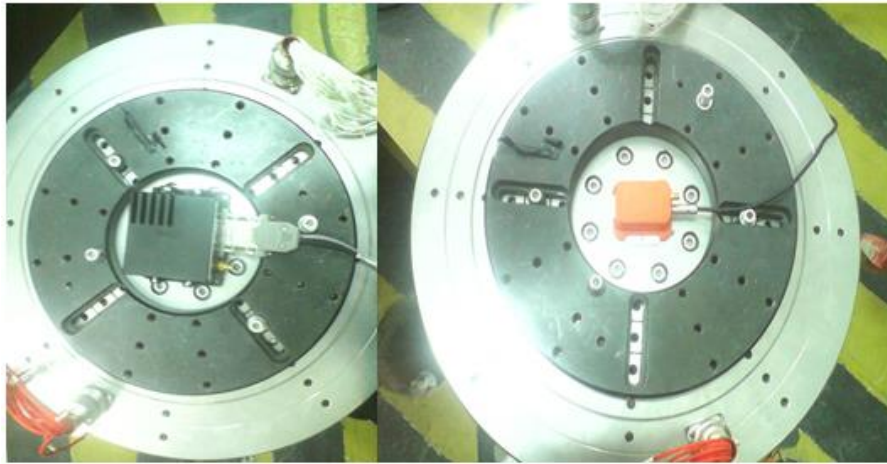
Figure 4.25 Installations of MEMS IMU on the single-axis rotation platform
