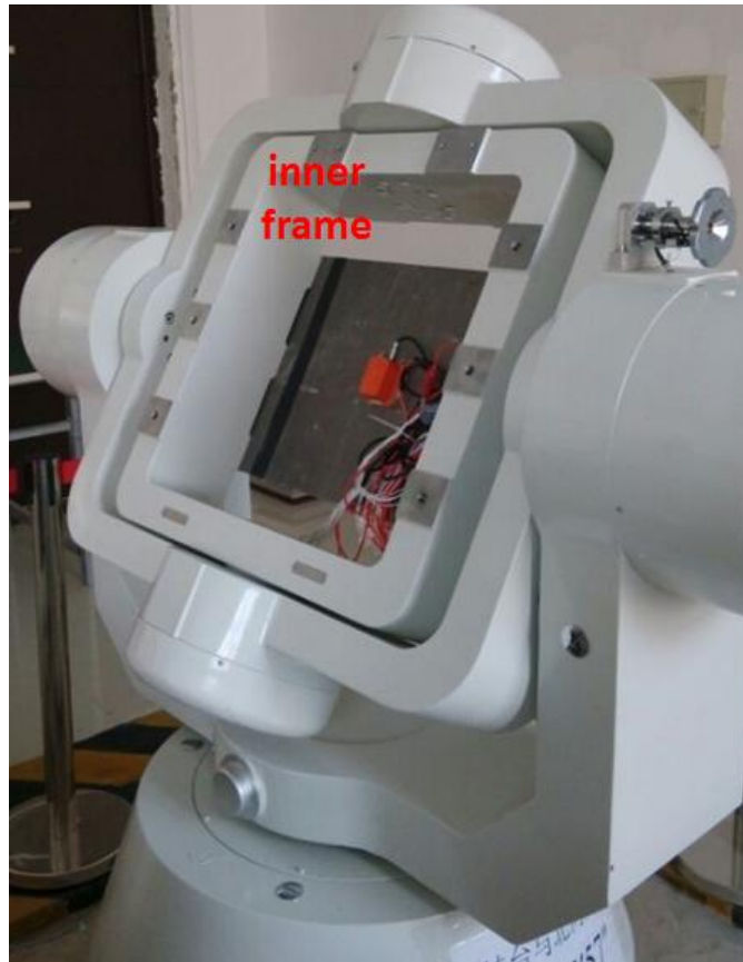
Figure 5.14 Rotation table set-up for IMU rotation about Z axis with middle frame at angle position of 60^\circ
