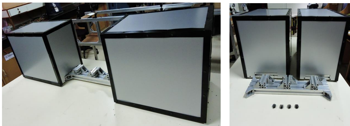
Figure 15: The supporting structural framework for housing NIR-IBBCEAS instrument. The separation between the transmitter and receiver units could be varied from 50 cm to 100 cm.
