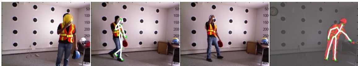
Figure 6.12: Sample image frames of hardhat classifier failures
