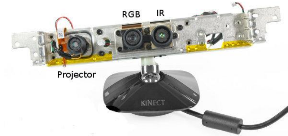
Figure 3.3: Kinect sensor composition
