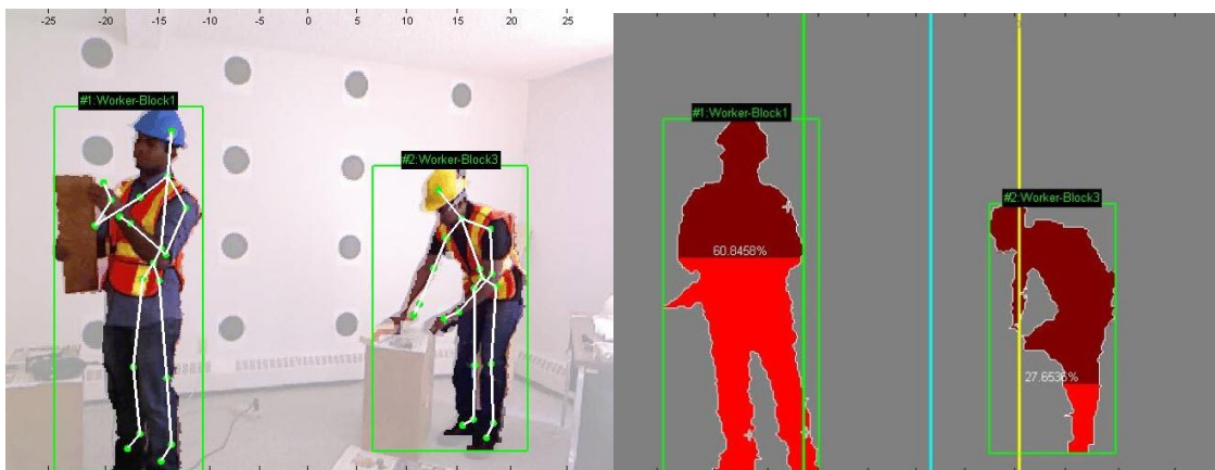
Figure 6.8: Background subtraction and tool-time indicator
