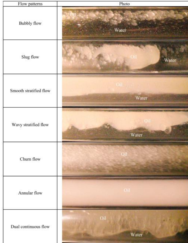
Figure 2.4. Photos of oil-water two-phase flow patterns in a 20 mm ID horizontal pipe (Hanafizadeh et al. , 2015).
