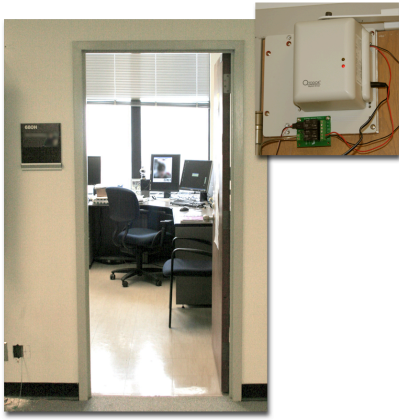
Figure 1. An overview of the office node of the ME-dia space, taken from just outside the teleworker's office. The inset photograph illustrates the motor mechanism used to open and close the office door remotely.
