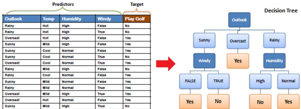
FIGURE 1.7. CONSTRUCTION OF A DECISION TREE USING WEATHER-BASED FEATURES (LEFT) IN ORDER TO PREDICT IF A PERSON WILL PLAY GOLF OR NOT. ( HTTP://WWW.SAEDSAYAD.COM/DECISION_TREE.HTM )
