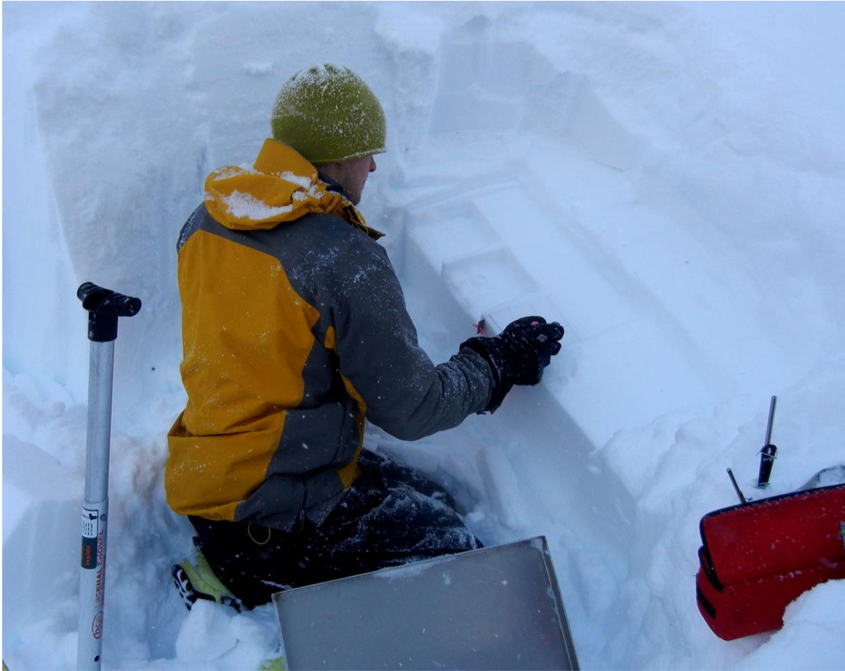
Figure 3.12: An example of shear frame tests during winter field work. Two tests have been completed and the author is preparing the third test.
