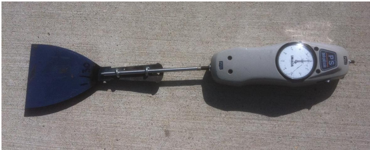
Figure 3.8: Basic equipment set-up for thin-blade resistance measurements is a force gauge with a custom blade attachment made from a 4" (~10 cm) paint scraper
