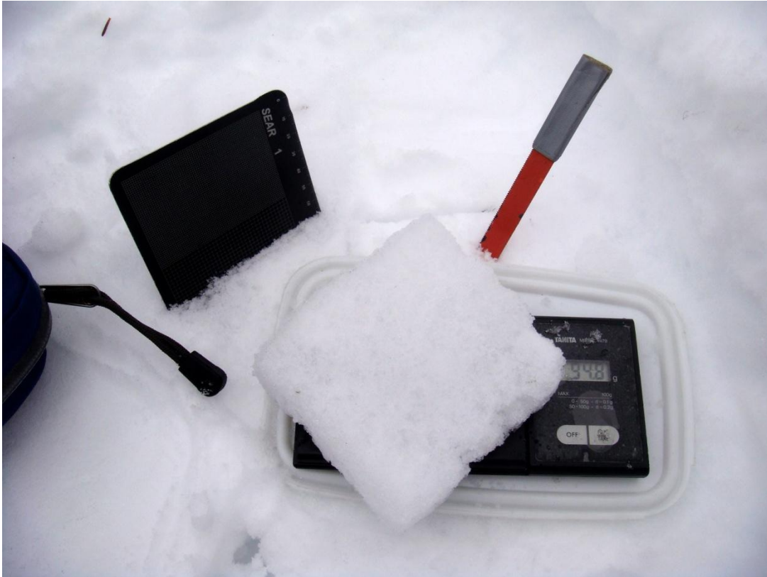
Figure 3.11: An example of a crust density measurement. A block of crust is isolated using a small saw and the three dimensions are measured and recorded. The mass of the block is measured using a small digital scale and the density can then be calculated. Three measurements were made for each observation to reduce uncertainty.
