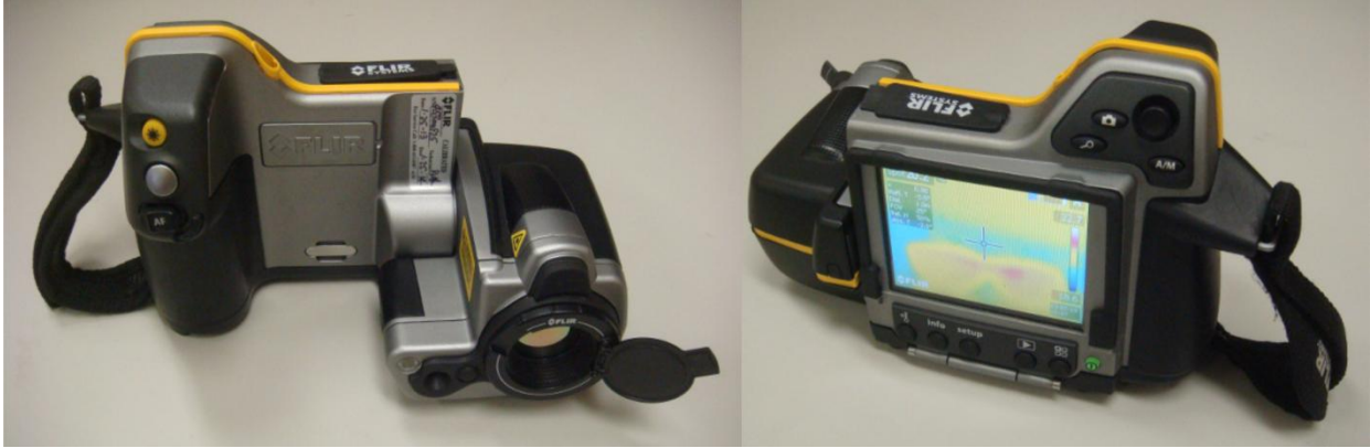
Figure 3.9: FLIR B300 thermal camera used for thermal imaging of melt-freeze crusts.
