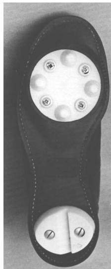
Figure 2-2: Photograph of the swivel disc shoe (Cameron & Davis 1973).
