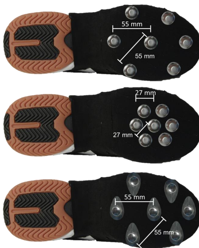
Figure 7-3. Photographs of the three footwear conditions, control (top), low rotation (middle) and high translation (bottom).
