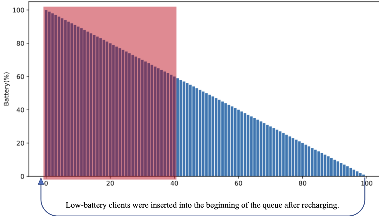
Figure A.1: Clients are queued according to their respective battery percentages. Only clients with sufficient battery levels are selected in each global epoch.
