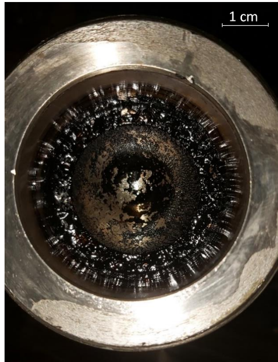
Figure 4.4: Heavy cut accumulated at the bottom of the equilibration cell after LLE experiment at 40 °C and 45 wt.% LPG in the feed.
