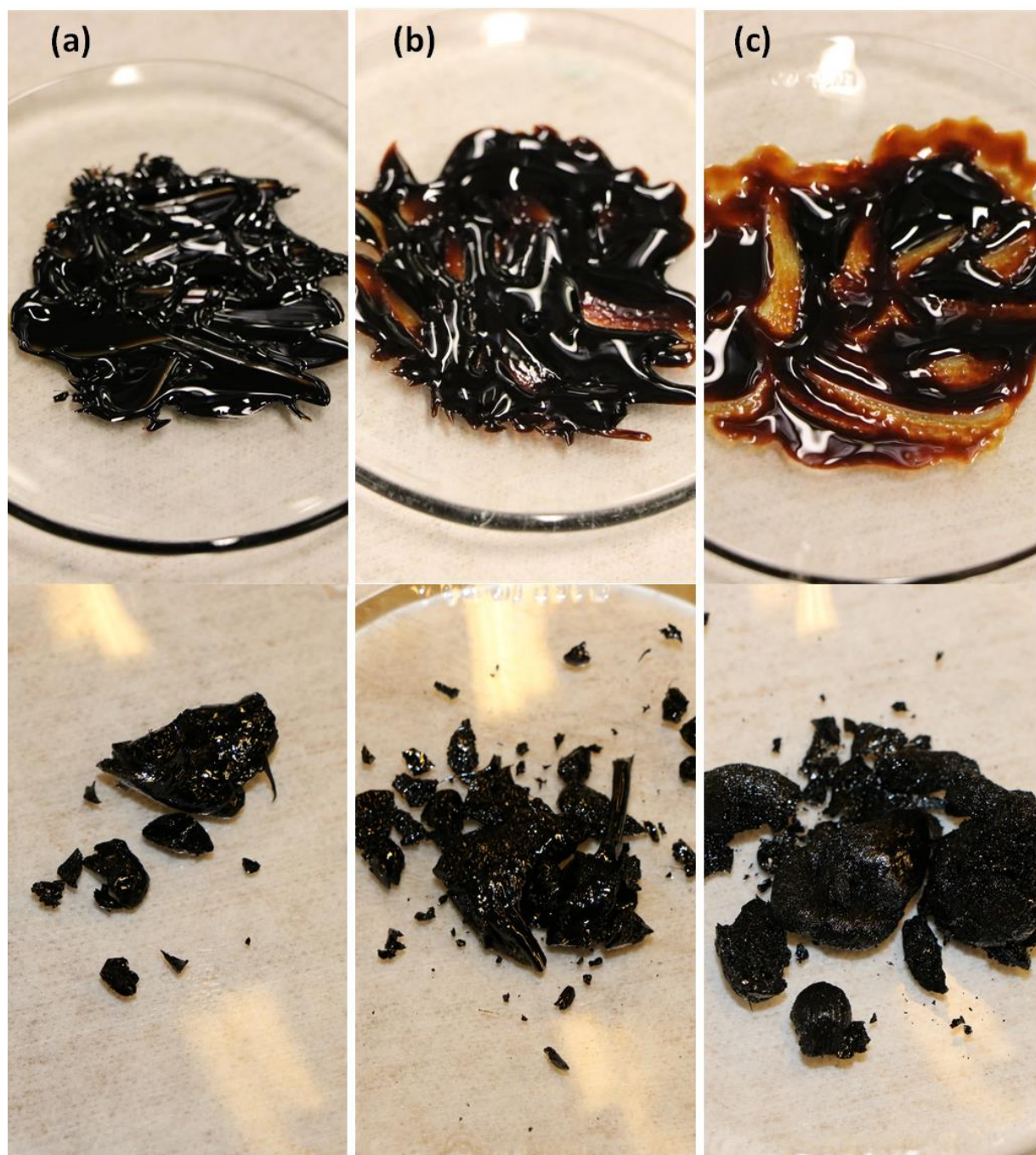
Figure 4.7: Light cuts and the corresponding heavy cuts from LLE of LPG/bitumen mixtures at 80 °C and solvent concentration of (a) 45, (b) 55, and (c) 65 wt.% in the feed.
