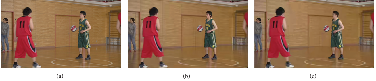
FIGURE 4: Frame from Basketballpass test video: (a) original video, (b) encoded video using existing HM encoder, and (c) encoded video using proposed DCT algorithm.
