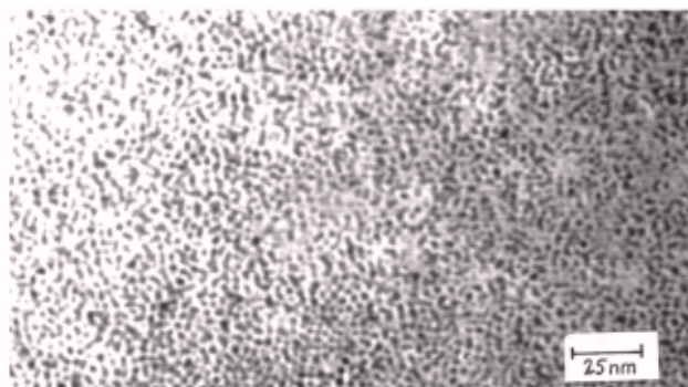
Figure 3. TEM view (530,000 times magnification) of Ir nanoparticles on plain Cu grid, formed by the SG technique, using a withdrawal rate of 1.2 cm/min and air-dried for 25 min. 100 kV accelerating voltage was employed.
