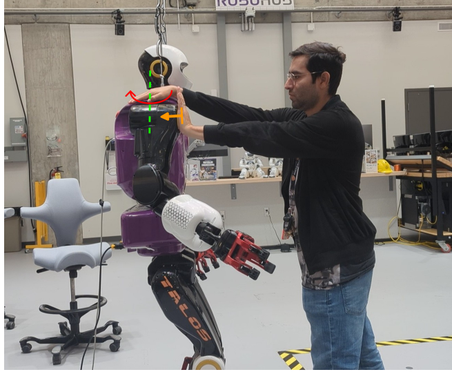
Figure 6.7: The TALOS Robot Experimental Setup. The orange arrow denotes the direction of the applied force. The green dotted line denotes the axis of rotation for the joint, whereas the red arrow shows the resulting joint movement.
