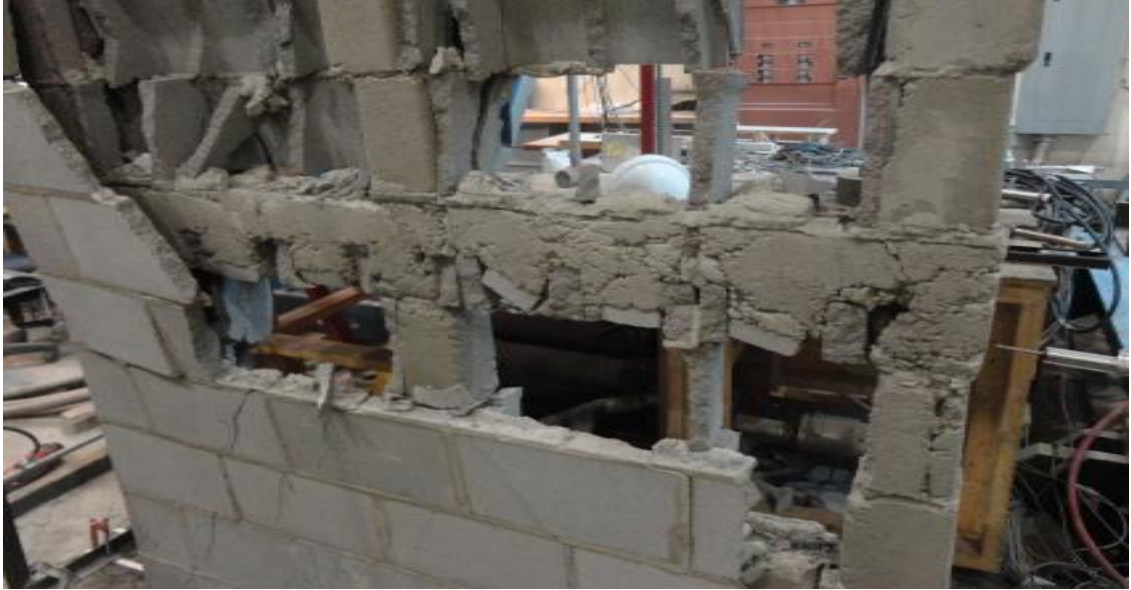
Wall 4-B (At the end of testing)
