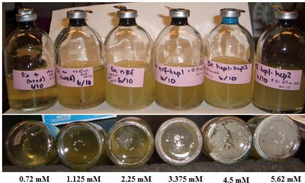
Figure 5.1 Increasing amounts of oxygen added to stationary phase D. vulgaris cultures containing 18 mM sulfide generated increasing amounts of PS. The cultures became visibly more turbid with more oxygen due to increased sulfur precipitate, which can be seen adhering to the bottom of the serum bottles (bottom panel). The R_{OS} from left to right are: 0.04:1, 0.0625:1, 0.125:1, 0.1875:1, 0.25:1, 0.31:1.
