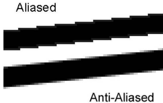
Figure 4.1 - Image quality due to aliasing
