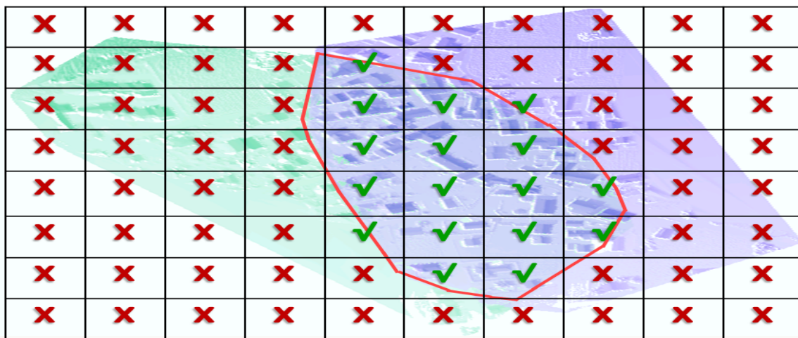
Figure 3.7. The selected overlapping region between two LiDAR strips (1&9) (✓)
