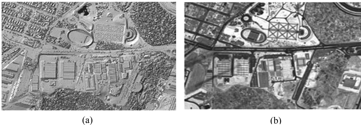
Figure 2.3. Sample of interpolated LiDAR imagery: (a) range image and (b) intensity image (Bossler, 2010)
