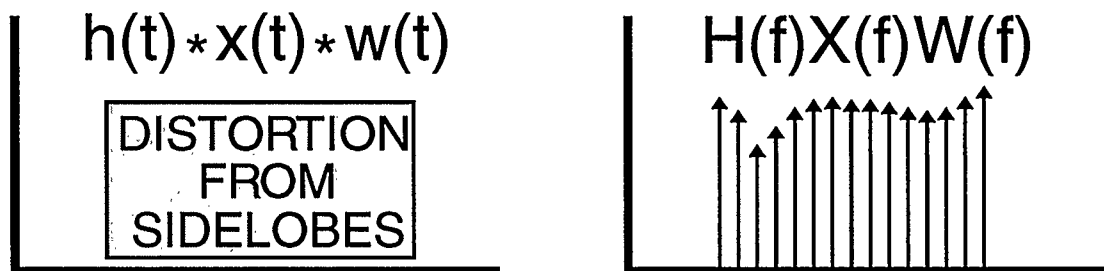
Figure 2.8e: Sampled, Band Limited Frequency Domain and Time Domain Representation
