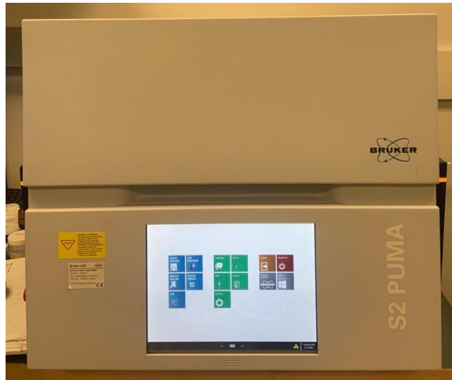
Figure 3.5: X-ray fluorescence (XRF) equipment
