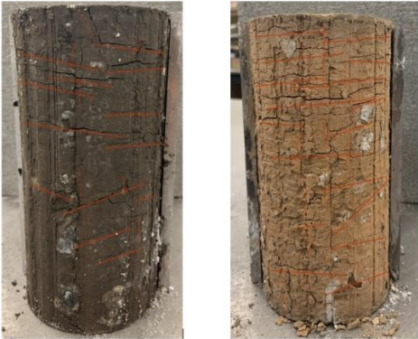
Figure 4.3: Crack identification of the sample before and after heating treatment
